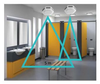
Sensor covers  $^{\sim}2 - 2.5$  meter radius zone. Best sensor mounting height is up to 3 - 3.5 meters.
