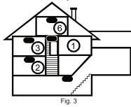
In multi-storey flats and family houses the detector should be installed above the stairs. It is recommended to place additional detectors in all rooms where people sleep. See Fig 3.
