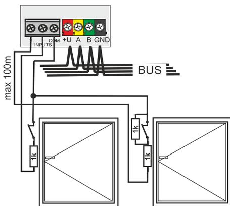
Figure 3: Loop balancing
