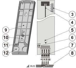
Fig 2: 3 - production number; 4 - antenna; 5 - tamper contact; 6 - BUS connector; 7 - attachable bus terminals; 8 – BUS cable; 9 – rear housing part; 10 – tampering detection segment 11 - cable separator; 12 - holes for BUS cable
